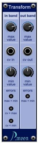
**Transform** is used to adapt a control voltage. It transforms a signal with a voltage between *Min1* and *Max1* to a signal with a voltage between *Min2* and *Max2*. Any voltage from -10 to +10 volts can be processed. If input voltage exceeds limits, it will be clipped at set limits. LEDs indicate error states. In case of error "max = min" output signal will be set to 0 volts.
