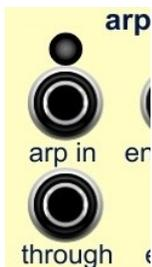
LED indicates an ON signal (< 2.5 V) at **arp in**.
