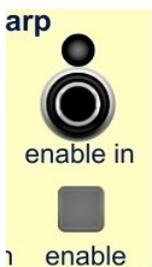
LED indicates an ON signal (< 2.5 V) at **arp enable in**.
