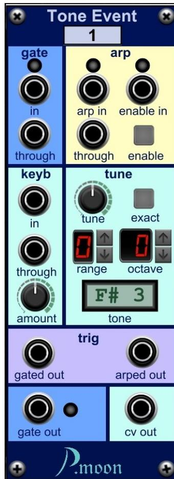
This module can be used both as standalone and as stage of a step sequencer. It provides GATE and CV output signals, that can be used to control any sound source. Together with a *P.moon* Stepper module several **Tone Event** modules can form a step sequencer.
