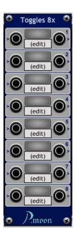
**Toggles 8x** can be used as CV source as well as signal switch. It contains eight toggle button sections:
