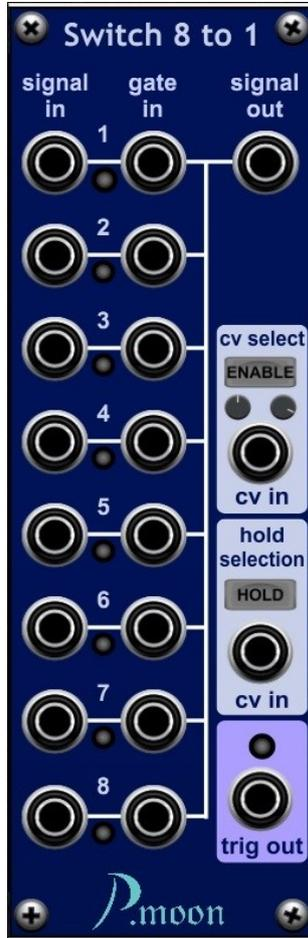
This module switches eight input signals to one output jack. Selection is done either by GATE signals or a CV voltage.
