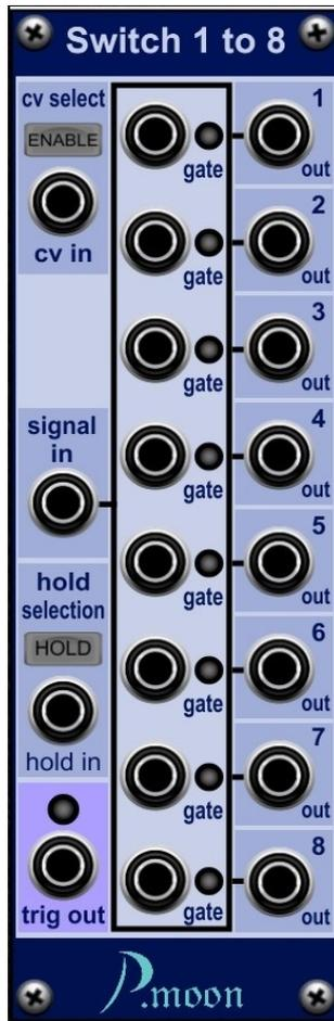
This module switches an input signal to one of eight output jacks. Selection is done either by **GATE** signals or a **CV** voltage.
