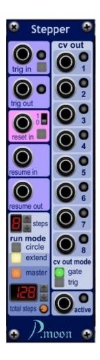
Together with **Tone Event** module this module can be used to build up a step sequencer. Several Steppers may be cascaded, even with less than 8 steps each.
