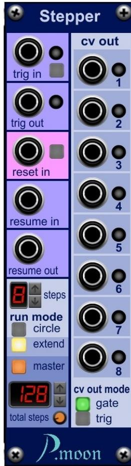
Together with **Tone Event** module this module can be used to build up a step sequencer. Several Steppers may be cascaded, even with less than 8 steps each.
