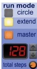
**Master** button should toggled on, when actual **Stepper** is the first one in a **Stepper** cascade.
