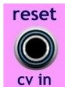
A pulse sets slope to zero instantly. Then operation continues as before reset.
