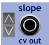
**Slope CV out** jack delivers slope voltage.
