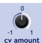
**CV amount** knob determines, how much voltage at **CV In** can influence slope time. Internally CV is normalized. That means, a CV from -5 to +5 equals a -1 to +1 value for calculation. This value is added to knob value.
