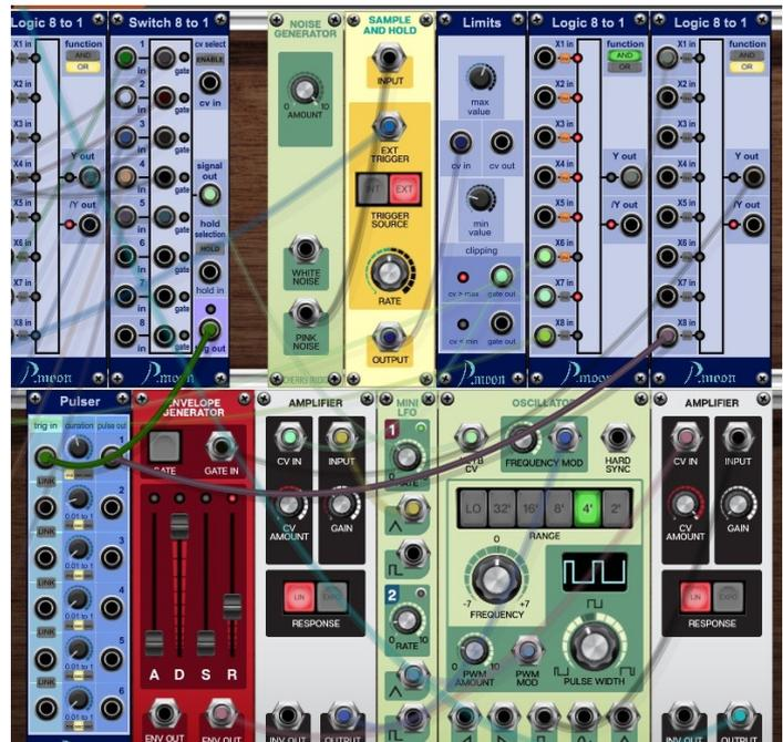
This short pulse will be enlarged by *Pulsar*. Please note, that enlarged pulse must be shorter than a *Stepper's* step. Otherwise it's output will stay ON continuously and ADSR will remain at "S" level.
