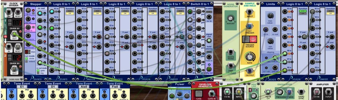
Second GATE part is made to get a ratcheting effect as "illustration". A *Voltage Noise Generator* and a *Voltage Sample and Hold* deliver the random CV. With *P.moon Limits* we can adjust, how often the effect is active. First *Clock Divider's* output will provide a double note at given steps.
