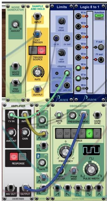
We don't want to get this effect during step 8, when no tone frequency is selected. With AND function of another *Logic 8 to 1* module and inverted step 8 "cv out" this problem is solved. Output of "Limits" goes also to a *Voltage Amplifier*. It controls frequency modulation of tone oscillator at same time, when a ratcheting effect happens.
