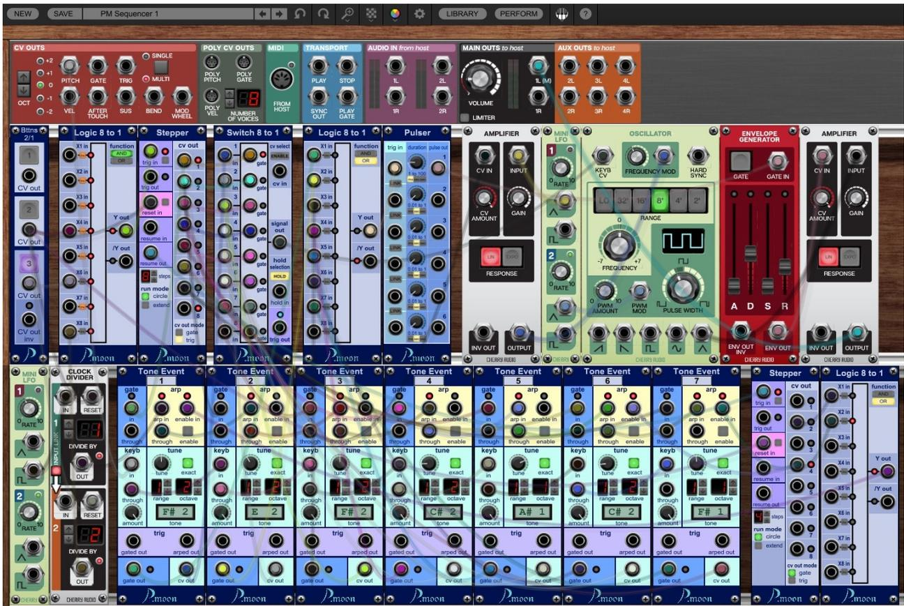
Each *Tone Event* creates both KEYB and GATE signals. Common step sequencers offer just one KEYB and one GATE output. Because this sequencer is modular, there is something to do for getting just this single KEYB and GATE outputs. Therefore additional *P.moon* modules are used as are *Switch 8 to 1* and *Logic 8 to 1*.
