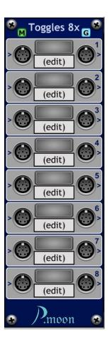
**Poly Toggles 8x** is intended to control up to eight poly signal channels by toggle buttons. A mute toggle button allows you to switch off all poly channels simultaneously. In gate mode each channel output can create a poly gate signal. Each label is editable after a double click on it.
