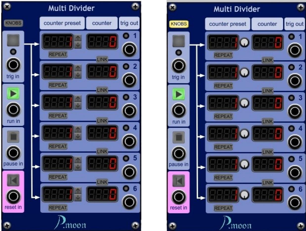
**Multi Divider** contains six equal channels that can be used to divide input frequency or to create trigger signals, when a distinct number of pulses is count. These counters may operate simultaneously or cascaded.
