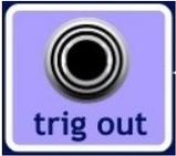
Each time, stage eight gets an ON value from stage seven, this jack sends a trig pulse of one sample length.
