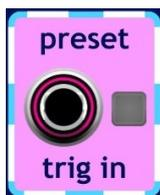
A trig pulse or a click onto the button will load start value into register.
