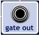
This gate out jack provides +5 volt, as long as register stage no. 8 is ON.
