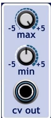
With **max** knob you can define highest cv out voltage at register value "**255**".
