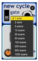
New cycle output provides a signal when a step cycle begins. With slide switch in gate position output voltage is +5 volt as long as sequencer is in step #1 (forward) or (count)# (reverse). LED is on at same time.
