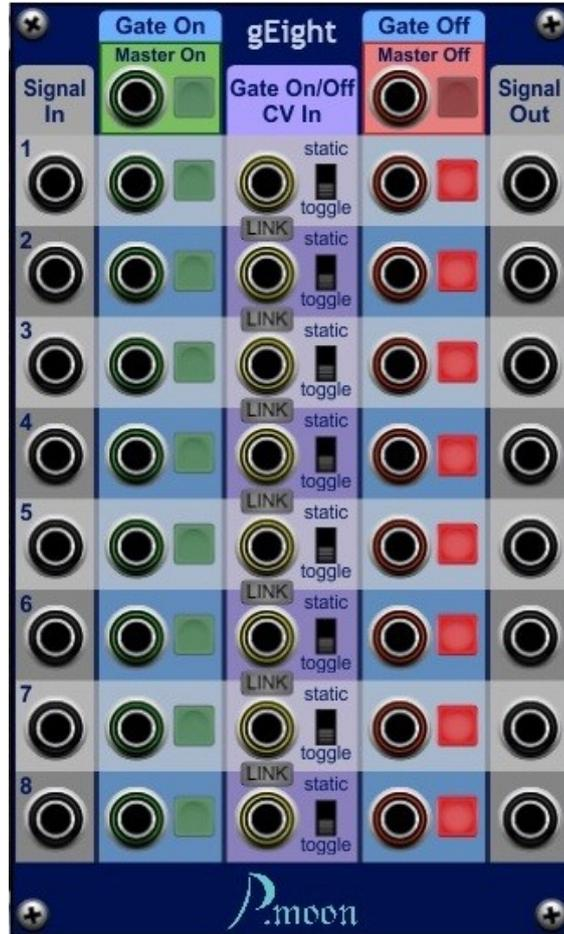
**gEight** contains eight equal signal gate channels which can be controlled by buttons or CV.
