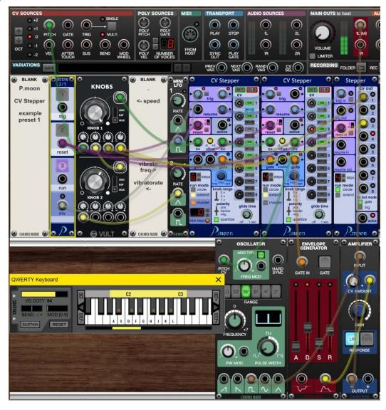
This is a typical preset with two cascaded **CV Stepper** modules, which work as 16 step sequencer. **Stepper** is used to change sequencer's basic tone.
