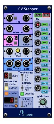
**CV Stepper** is an improved variant of **Stepper**. With added CV knobs, it can deliver a different voltage at each step. Additionally it has got a glide function. It works even triggered with audio frequencies. So it can be used as stepped wave form oscillator too.
