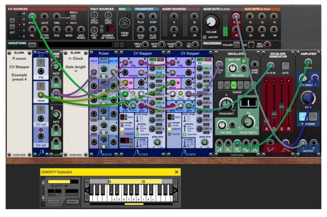
In this preset common sequencer consists of two **CV Stepper**s too. But here **enable** inputs are used at **CV Stepper** modules. This way **gate** output pulses length can be controlled by input **enable** pulse length. A **P.moon Pulser** provides this changeable pulse length.
