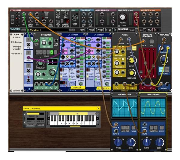
In this preset there is also a 16-step sequencer. But this time it is triggered by a high audio frequency. Now sequencer's CV output voltage is not used to modulate an oscillator, it IS an oscillator output signal.
