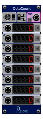
**OctoCount** contains 16 digital counters, separated in two groups. Lower group (channel 1 to 8) is equipped with mono input sockets and with red displays. Upper group (channel 9 to 16) can only used with poly input connector. Their displays are green.
