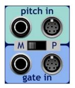
Connect cables for pitch and gate to these sockets. You can use both mono and poly connectors at same time.
