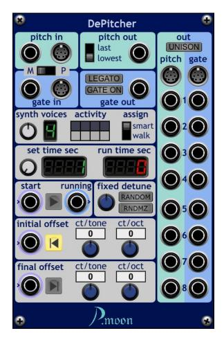
This module is intended to simulate inaccurately tuned voices of ancient analog synthesizers and it's long time frequency drifting as a result of thermal influences.
